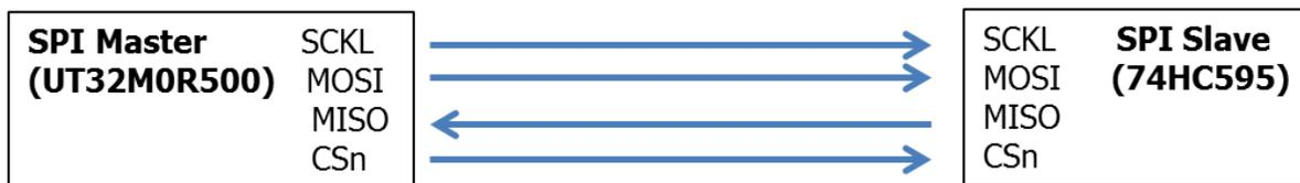
**Figure 1: SPI master/slave communication**
