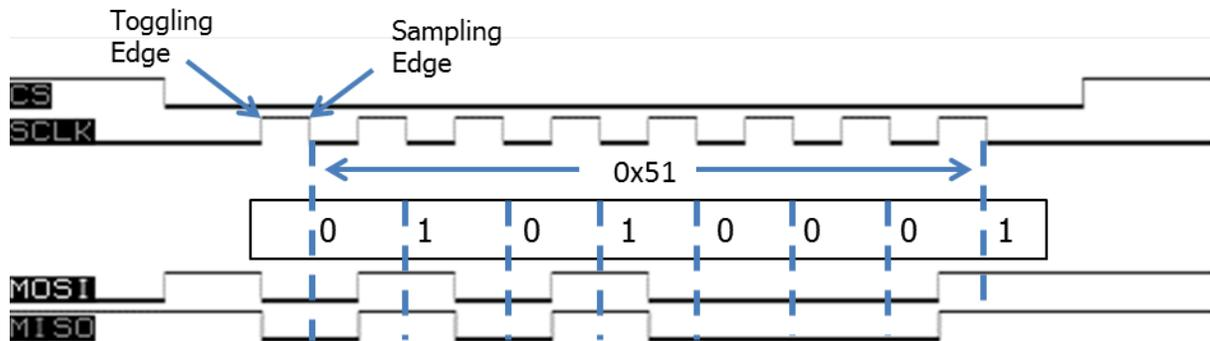
Figure 6: SPI Master/74HC595 Slave Mode 1 Configuration
