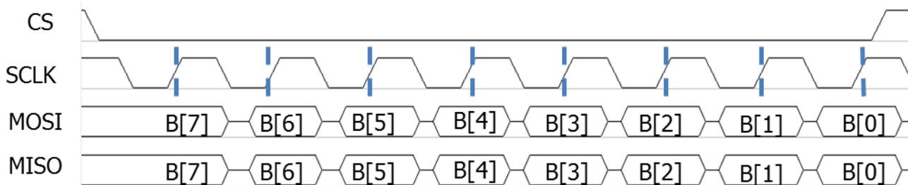
**Figure 5: Master and Slave Communication with Mode 0**
