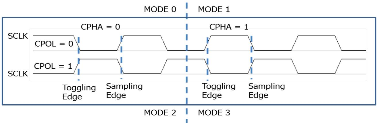
Figure 2: Clock Polarity and Clock Phase Configuration
